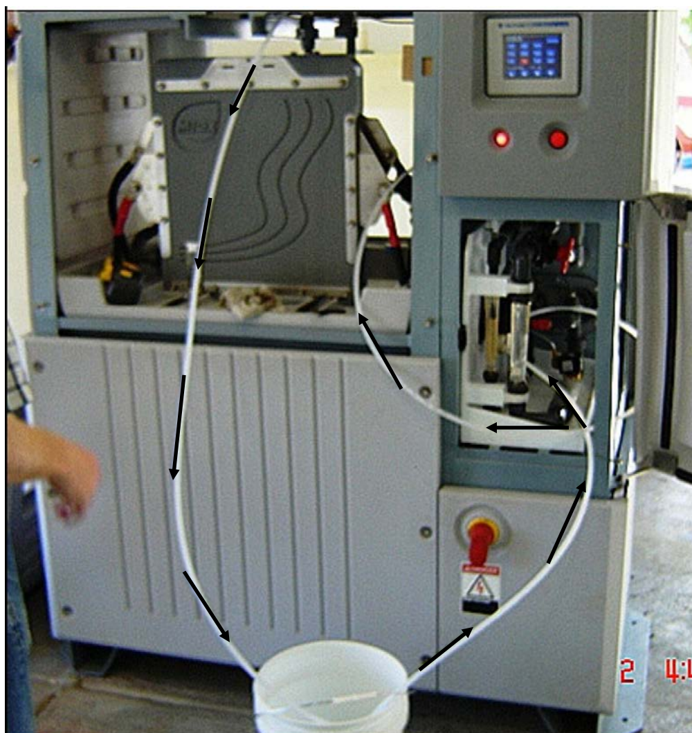
Figure 4 Acid Wash Recirculation Set Up
